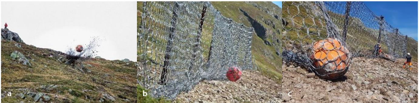
Figure 1: a: rockfall impact on the ground after release; b: eccentric rockfall impact in the netting; c: inspection of the barrier after consecutive impacts
