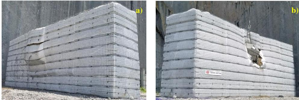
**Figure 1: Deformed shape of the embankment after the impact: a) downhill face; b) uphill face**
